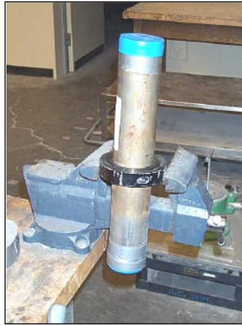
Figure 12: Shelby tube with stiffener ring to prevent tube distortion
