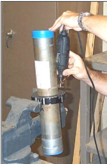
Figure 13: Cutting Shelby tube with low-vibration, high-speed rotary cutting tool
