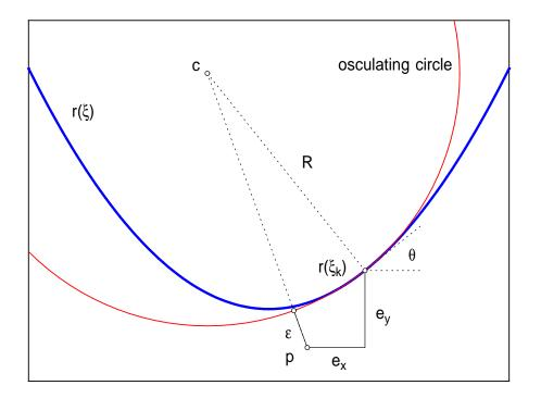
quasi-linear contour error estimate  $\epsilon \approx -C_x e_x + C_y e_y$  by approximation of the curve with circle of curvature at  $\mathbf{r}(\xi_k)$  — where the "variable gains"
