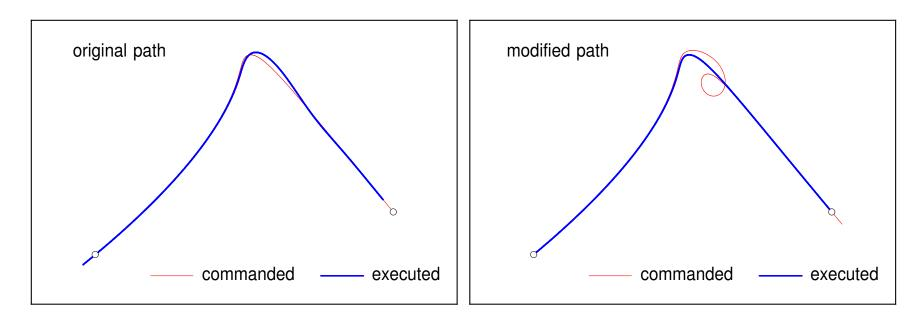
Comparison of commanded and executed motions for original (left) and modified (right) paths. In the former case, the executed motion deviates significantly from the desired path. In the latter case, the executed motion is essentially indistinguishable from the original commanded path.
