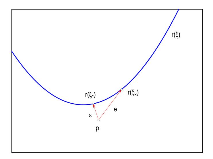
$\mathbf{r}(\xi_k) = \text{reference point}$  (commanded position) and  $\mathbf{p} = \text{actual position}$ (measured by encoders) at  $t_k = k \Delta t$ . Then position error  $\mathbf{e} = \mathbf{r}(\xi_k) - \mathbf{p}$ and contour error  $\boldsymbol{\epsilon} = \mathbf{r}(\xi_*) - \mathbf{p}$ , where  $\mathbf{r}(\xi_*)$  is the *footpoint* of  $\mathbf{p}$  on  $\mathbf{r}(\xi)$ .
