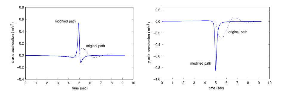
Comparison of x and y axis accelerations for original and modified paths. The modified path incurs greater peak accelerations, requiring a higher motor torque capacity.
