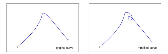
Left: quintic PH curve defining desired path  $(X(\xi), Y(\xi))$ . Right: modified path  $(\hat{X}(\xi), \hat{Y}(\xi))$  that compensates for the machine/controller dynamics, for a P controller with gain  $k_p = 10$  and constant feedrate V = 0.12 m/s.
