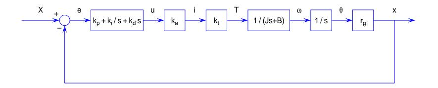
X = commanded position from real-time interpolator x = actual position as measured by position encoders e = X - x = instantaneous *x*-axis position error  $k_p, k_i, k_d =$  proportional, integral, derivative gains u = output voltage from controller i = current from current amplifier T = torque from DC electric motor J, B = x-axis inertia and damping  $\omega, \theta =$  motor shaft angular speed & position  $r_q =$  transmission ratio (angular  $\rightarrow$  linear conversion)
