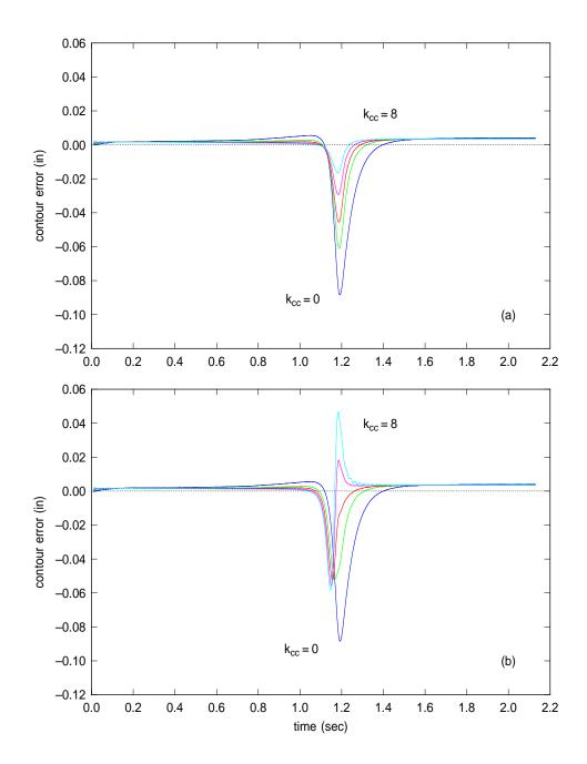
measured contour errors using exact computation (upper) and osculating circle approximation (lower) with cross-coupling gains  $k_{cc} = 0, 1, 2, 4, 8$ .
