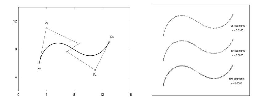
Left: analytic tool path description (quintic PH curve). Right: approximation of path to various prescribed tolerances using piecewise-linear G codes.
