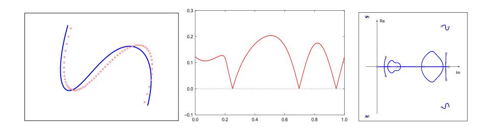
left: quintic curve  $\mathbf{r}(\xi) = (x(\xi), y(\xi))$  with discrete sampling of machine positions  $\mathbf{p} = (x_p, y_p)$ ; center: contour error of machine positions  $\mathbf{p}$  with respect to  $\mathbf{r}(\xi)$ ; right: variation of roots of the polynomial  $F(x_p, y_p, \xi) = 0$  in the complex plane as  $\mathbf{p}$  moves.
