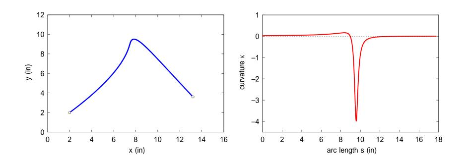
left: PH quintic test curve used in cross-coupled controller experiments; right: curvature profile — showing sharp curvature "spike" — of test curve
