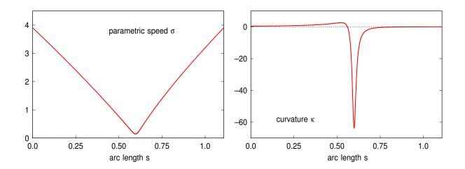
Extreme variation of parametric speed and curvature on quintic PH curve.
