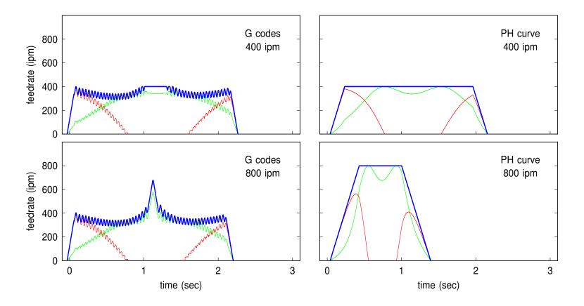
At 400 & 800 ipm, the PH curve interpolator continues to yield impeccable performance – but the performance of the G code interpolator is severely degraded by "aliasing" effects, incurred by the finite sampling frequency and discrete nature of the piecewise-linear path description.
