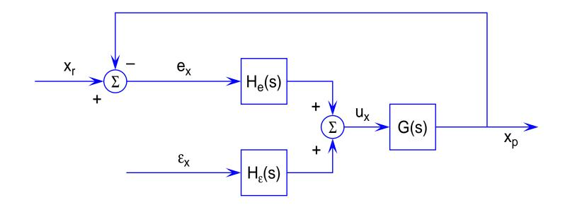
actuating signal for the *x*-axis is a combination of the position error  $e_x$ and contour error  $\epsilon_x$  components, as modulated by individual (e.g., PID) controller transfer functions  $H_e(s)$  and  $H_{\epsilon}(s)$
