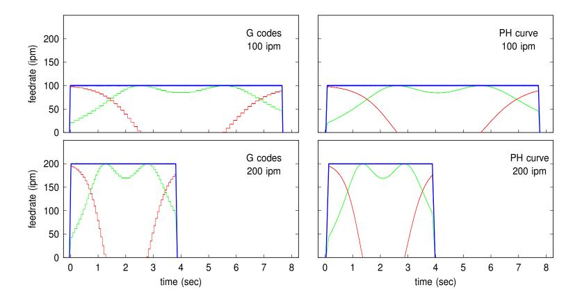
The G code and PH curve interpolators both give excellent performance (red) at 100 and 200 ipm. The "staircase" nature of the x and y feedrate components (blue and green) for the G codes indicate faithful reproduction of the piecewise-linear path, while the PH curve yields smooth variations.
