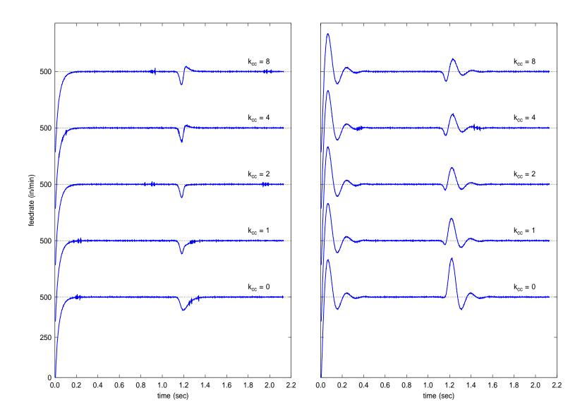
measured feedrate (for a 500 in/min command rate) with cross-coupled P (left) and PI (right) controllers, using exact contour error computation
