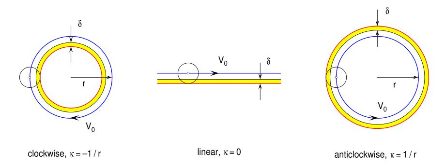
Volume removed (yellow area) by a cylindrical tool of radius d moving with feedrate  $V_0$  through depth of cut  $\delta$  for: a clockwise circular path of radius r (left); a linear path (center); and an anti–clockwise circular path of radius r (right). In each case, the MRR can be expressed in terms of the curvature as  $V_0 \delta [1 + \kappa (d - \frac{1}{2}\delta)]$ . Hence, to maintain constant MRR, one should use the curvature–dependent feedrate
