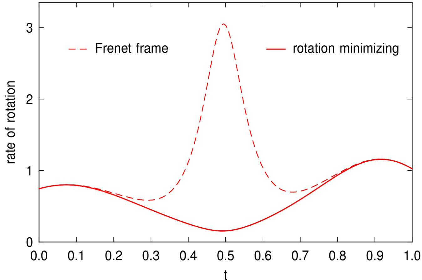
compared with the **rotation-minimizing frame**  $(\mathbf{t}, \mathbf{u}, \mathbf{v})$ , the **Frenet frame**  $(\mathbf{t}, \mathbf{n}, \mathbf{b})$  exhibits a lot of “unnecessary” rotation (in the curve normal plane)
