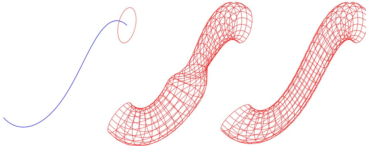
surface constructed by sweeping an ellipse along a space curve using Frenet frame (center) & rotation-minimizing frame (right)
