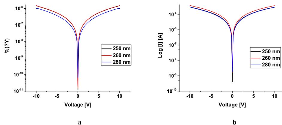
**Figure 13.** (a) semi-logarithmic plot of current–voltage for Au/ $\beta$ -Ga<sub>2</sub>O<sub>3</sub>/Au MSM with UV illumination at 10 V at different wavelengths such as 250 nm, 260 nm and 280 nm. (a) without catalyst (b) with Ag catalyst.
