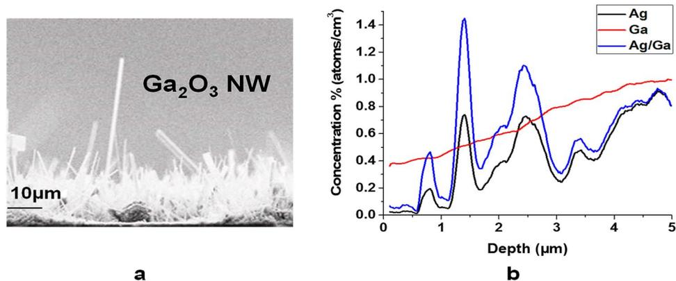
**Figure 5.**  $\text{Ga}_2\text{O}_3$  NWs on quartz substrate by 5 nm Ag catalyst at 1000 °C. (a) SEM image. (b) SIMS profile. The SIMS was performed for nanowires from the tip to the base. As we go from the tip to the root of NWs, the concentration of Ag increases.
