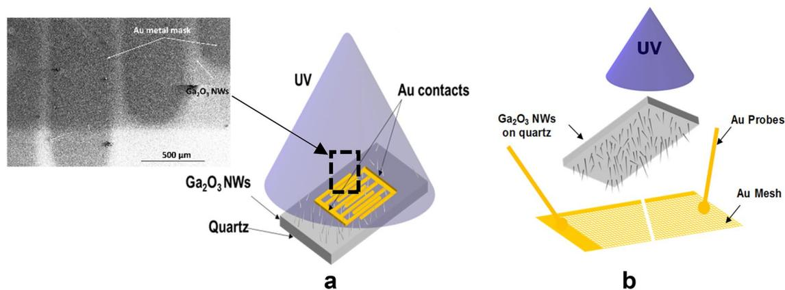
**Figure 11.** Schematic of Au/ $\beta$ -Ga<sub>2</sub>O<sub>3</sub>/Au metal–semiconductor–metal (MSM) photoconductor on quartz. (a) Sputtered gold contacts. The distance between the circles probes is 3 mm. Top-left SEM image of Au contacts at the surface of Ga<sub>2</sub>O<sub>3</sub> NWs. (b) Au mesh gold contacts.
