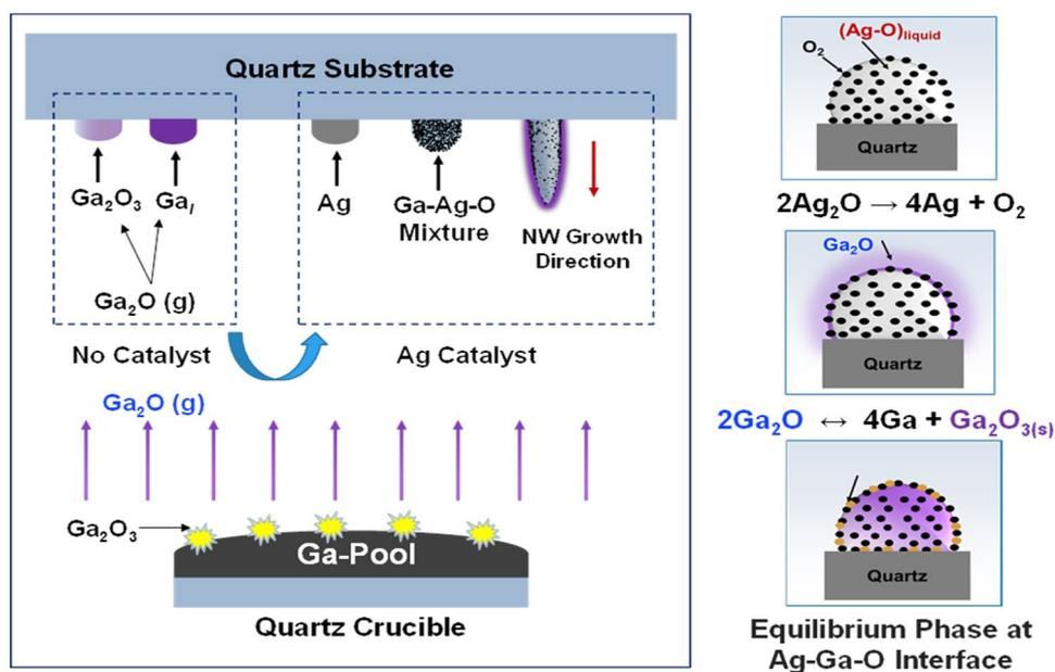
**Figure 16.** The growth mechanism of Ga<sub>2</sub>O<sub>3</sub> NWs on a quartz substrate coated with 5 nm Ag film (facing downward). A pool of liquid Ga is heated in a quartz crucible that sits under the quartz substrate with ~10 mm gap.
