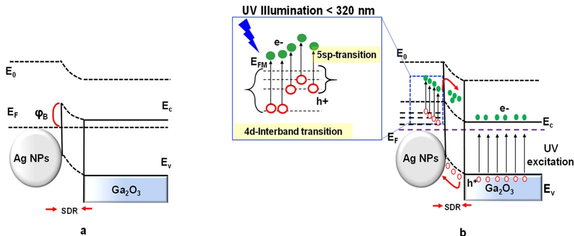
**Figure 17.** Energy band diagram at the interface of Ag NPs and Ga<sub>2</sub>O<sub>3</sub> NWs. **(a)** In dark condition, a localized Schottky barrier exists due to the difference in work-function. **(b)** Under UV illumination, the interband transition in Ag NPs enhances the photosensitivity of the UV detection and more photo-generated holes of Ga<sub>2</sub>O<sub>3</sub> NWs migrate to the surface by band bending.
