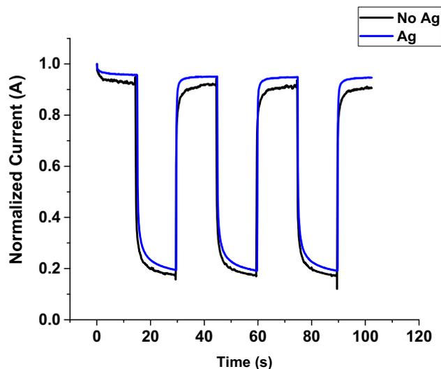
**Figure 15.** Transient response of the UV photodetector fabricated based on Au/ $\beta$ -Ga<sub>2</sub>O<sub>3</sub>/Au MSM at 5 V without and with Ag catalyst.
