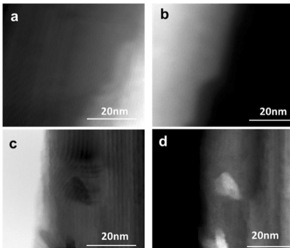
**Figure 6.** STEM images of  $\text{Ga}_2\text{O}_3$  nanowire growth on quartz substrate at 1000 °C. (a) Bright field (BF) (b) high-angle annular dark-field (HAADF) STEM images of  $\text{Ga}_2\text{O}_3$  nanowire without Ag catalyst. (c) Bright field (BF) (d) high-angle annular dark-field (HAADF) images of Ag NPs at the interface of  $\text{Ga}_2\text{O}_3$  nanowire. The nanoparticle was bright due to z-contrast.
