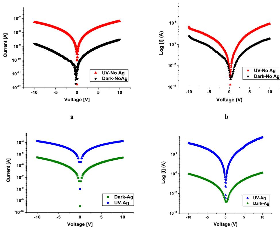
**Figure 12.** Semi-logarithmic plots of current density for Au/ $\beta$ -Ga<sub>2</sub>O<sub>3</sub>/Au MSM without and with Ag catalyst versus applied voltage characteristics at 10 V without and with UV illumination. (a,c) with sputtered Au metal contacts (b,d) with mesh Au metal contacts.
