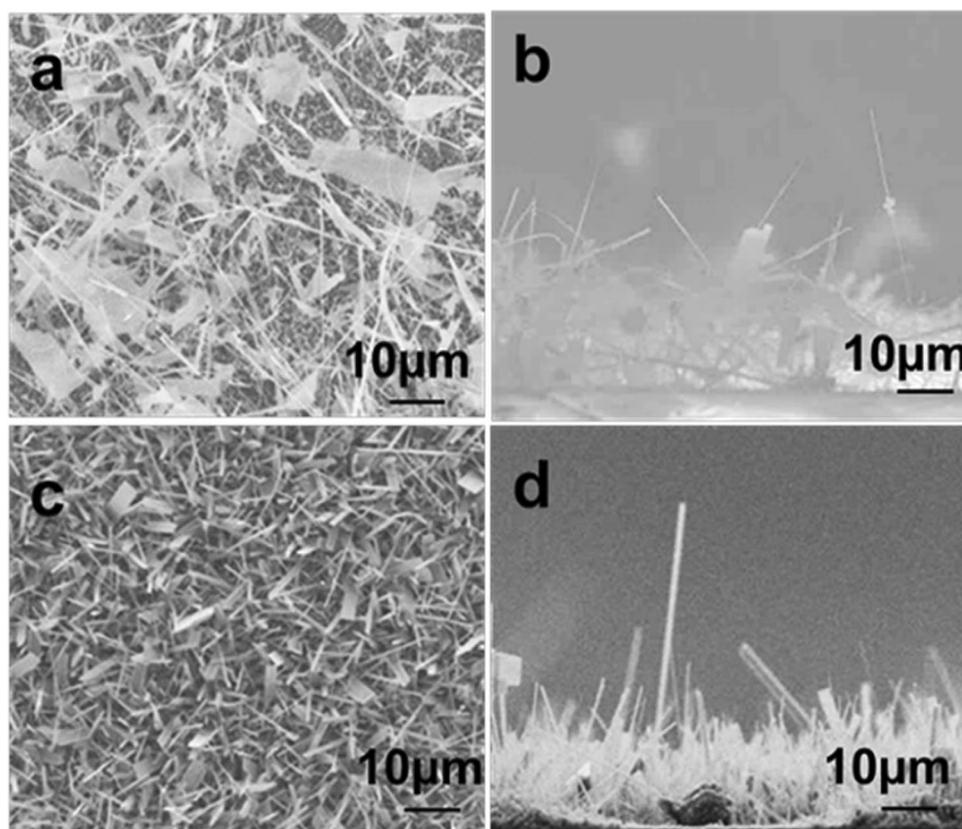
**Figure 2.**  $\text{Ga}_2\text{O}_3$  nanowire grown at  $1000^\circ\text{C}$ . (a,b) Top and side views of  $\text{Ga}_2\text{O}_3$  on a quartz substrate, respectively. (c,d) Top and side views of  $\text{Ga}_2\text{O}_3$  on quartz catalyzed by 5 nm Ag, respectively. Longer and denser NWs were achieved when Ag films are present on the sample before growth.
