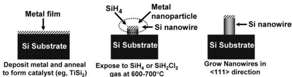
FIGURE 1 Schematic illustration of metal-catalyzed nanowire growth using chemical vapor deposition. A small metal nanoparticle accelerates the decomposition of a silicon-containing gas; the silicon atoms precipitate between the nanoparticle and the substrate, forming a column of silicon
