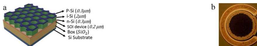
Fig.1 a) Proposed SiPD structure integrated with nanohole surface structure, b) Fabricated 30 \mu m diameter SiPD on SOI (Silicon-on-Insulator) wafer used for EQE and high-speed measurement.
