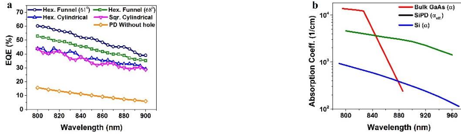
Fig.2 : a) Measured EQE Vs. wavelengths in SiPDs with micro/nano holes, b) Absorption coefficient in SiPD, bulk Si, and GaAs.
