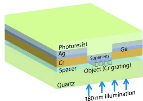
FIG. 1. (Color online) Schematic drawing of a smooth silver superlens with embedded 30 nm chrome gratings on a quartz window, operating at 380 nm wavelength. To prepare the smooth superlens, a thin germanium layer is seeded.
