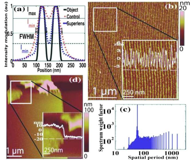
FIG. 3. (Color online) (a) Computed image modulation with superlens  $\text{FWHM}=37$  nm (blue dashed curve) and without superlens  $\text{FWHM}=113$  nm (red dotted curve). (b) Subdiffraction optical imaging with superlens: AFM of developed photoresist with zoom in panel showing section analysis. (c) Fourier analysis of the developed image grating. (d) Near-field optical imaging without superlens.
